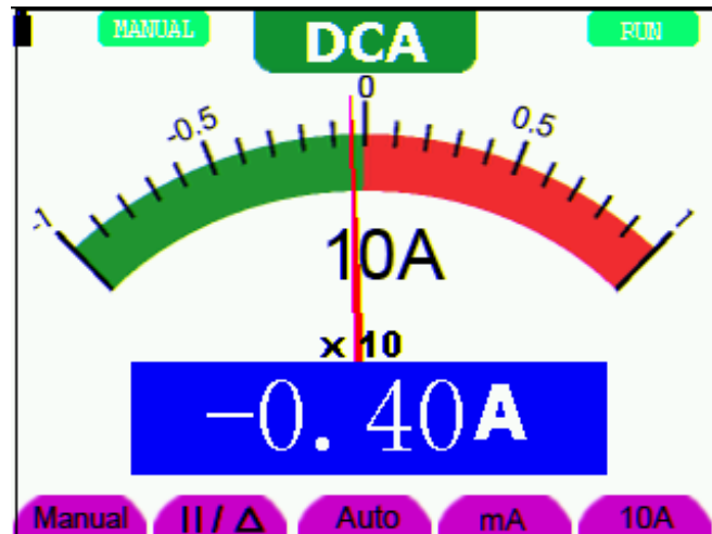
Figure 25: DC Current Measurement for 10A
